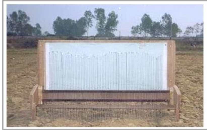
Figure 2. Surface roughness profiler for measuring the rms soil surface roughness in fields
